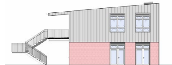
Above: Painted fibre cement Below: Veneer brick cladding
