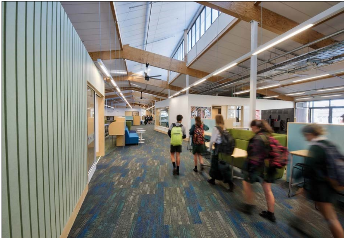
Figure 22: High ceiling and central clerestory rooflight.
