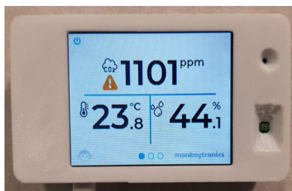
Figure 7: Example multi-element internal environmental monitoring device (data logger)
