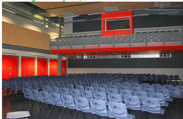
Figure 14: Secondary school hall with mechanical ventilation to mitigate outside traffic noise and providing the ability to mix air sources to minimise stratification effects in the high spaces.
