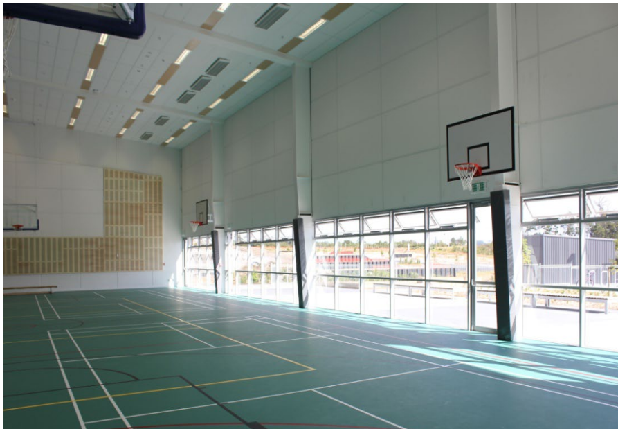
Figure 15: School gymnasium with openable windows for natural ventilation
