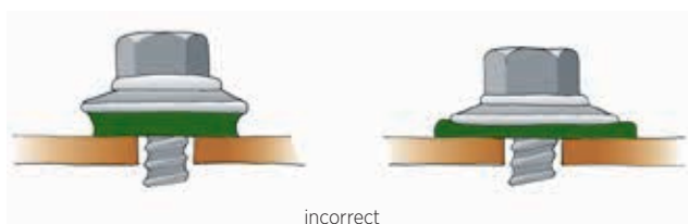
Tightening of roof fixings.
